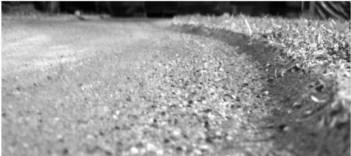
Figure 8. View looking downstream after Run 6.3. Coarser sediments transported and deposited along the channel thalweg (center of image) while finer sediments were selectively transported to and deposited on the bar (left side of image).
