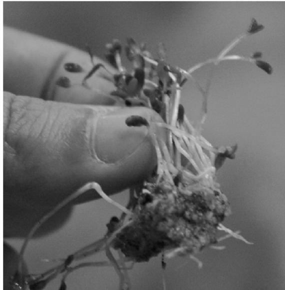
Figure 3. Alfalfa sprouts used to provide bank strength. Sand particles (model gravel) are cohesively attached to sprout roots.
