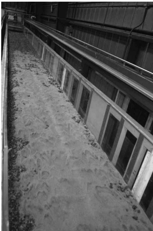
Figure 4. Photograph of the sand deposit prograding downstream over the gravel bedded channel for Run 2 at 4 h 15 min run time. Photograph is looking downstream. Note that the sand deposit has not covered the bed along the left wall in this picture.
