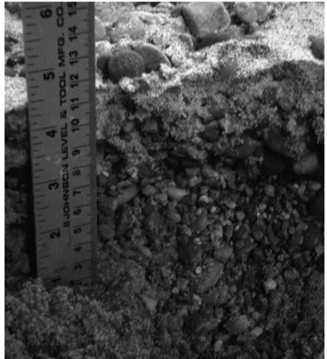
Figure 15. Photograph of the sediment deposit from Zone 5 at the termination of Run 1, illustrating the limited fine sediment infiltration depth. Ruler scales are inches (left) and centimeters (right).
